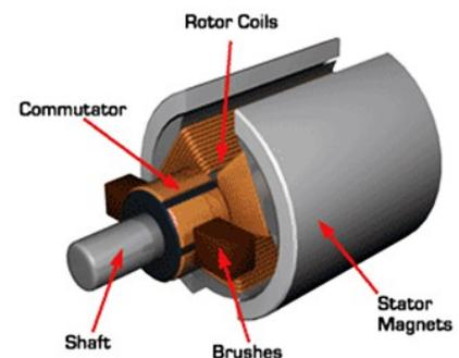
This motor types are not installed in new vehicles mostly because of their energy efficiency, which is around 75-80%. Brushes need to be replaced every 50kkm.
