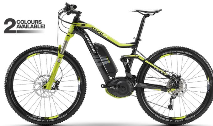
These electrically assisted bikes engine powers are moving typically 250W- 500W and the operating range of 30 to 80 kilometers.
